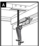
A: Start by pulling down latch handle from the back of cover. Then unscrew the handle to lower its position.
