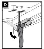
D: Latch the jaw groove fully into the rail lip, then crank handle down to tighten. Go back and readjust jaw position from step b if the latch does not feel very tight.
