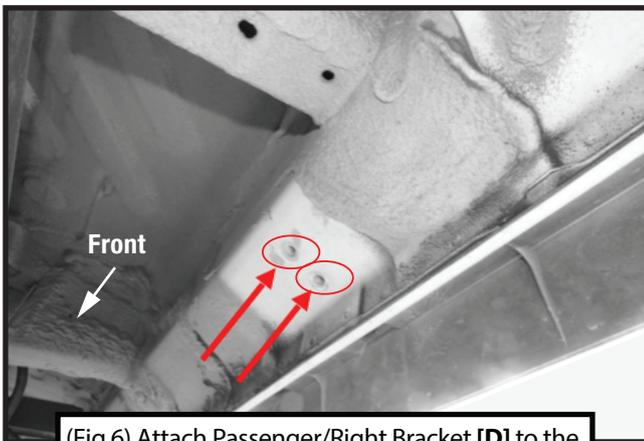
(Fig 6) Attach Passenger/Right Bracket [D] to the Passenger/Right side third mounting location
