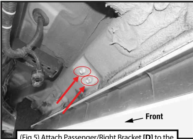
(Fig 5) Attach Passenger/Right Bracket [D] to the Passenger/Right side second mounting location (remove factory studs if necessary)
