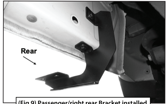
(Fig 9) Passenger/right rear Bracket installed
