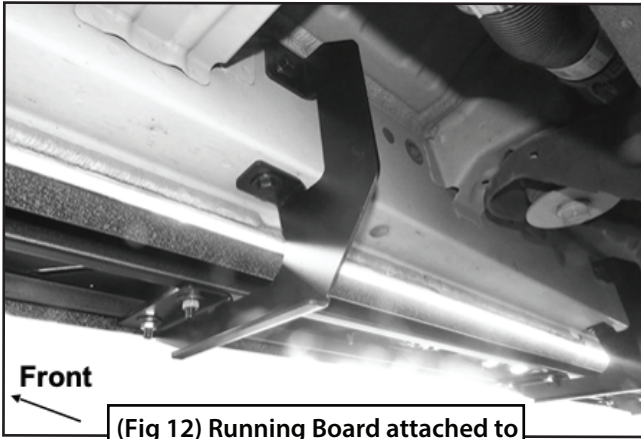
(Fig 12) Running Board attached to #2 and #3 Mounting Brackets
