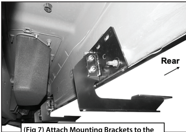
(Fig 7) Attach Mounting Brackets to the passenger/right center and rear locations
