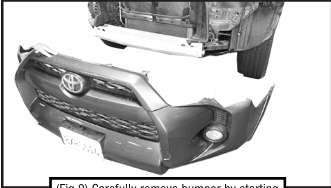
(Fig 9) Carefully remove bumper by starting at sides and moving towards center
