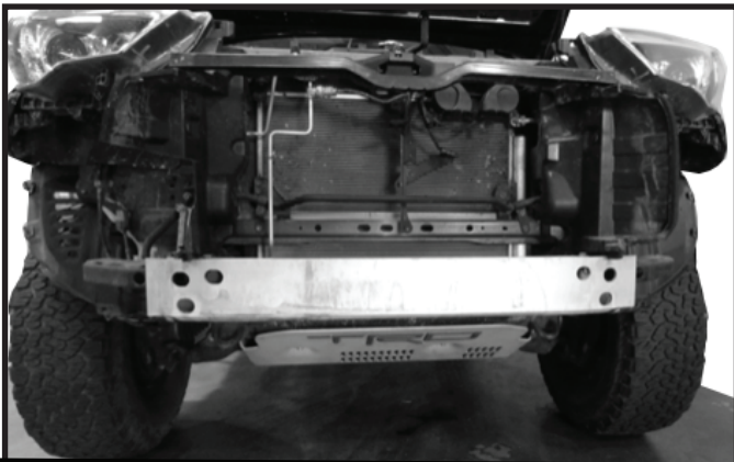
(Fig 10) Remove crash bar and frame extensions by uninstalling four factory bolts from the bracket face plate shown in (Fig 13)
