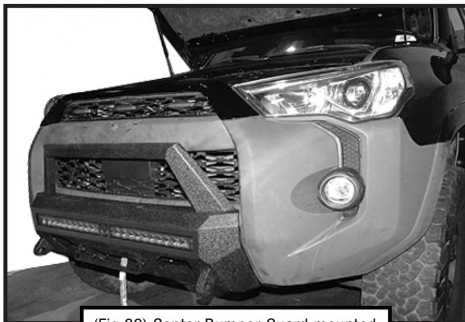
(Fig 39) Center Bumper Guard mounted
