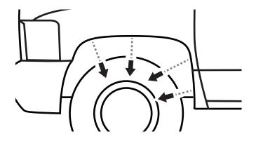
(1) Using a 7 mm socket wrench, remove 4 factory screws.
