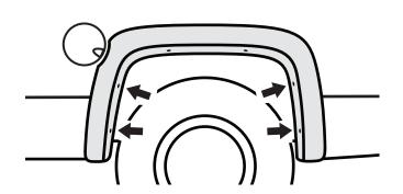
(8) Install 4 supplied PH Metal Screws **[E]** through remaining holes in flare and into S-clips installed in Step 6. Ensure proper flare fitment, then tighten all screws.
