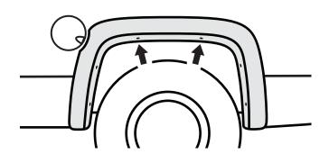
(7) Reposition flare. Install 2 supplied PH Truss Tap Screws **[D]** through top 2 holes in flare, into U-clips installed in Step 4, and into vehicle's factory holes. Do not tighten.
