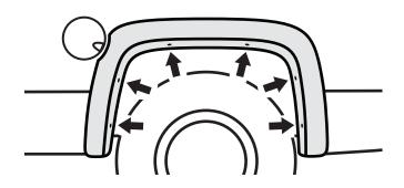
(3) Hold flare in position, with a grease pencil, mark 6 locations using holes in flare as guide. Then, remove flare.
