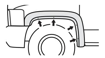
(2) Hold flare in position, reinstall 4 factory screws. Ensure proper flare fitment, then tighten all screws.
