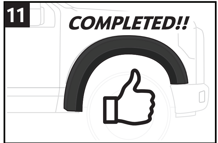
11. Tighten all screws. Repeat STEPS 1 to 10 to install the driver side front flare.
