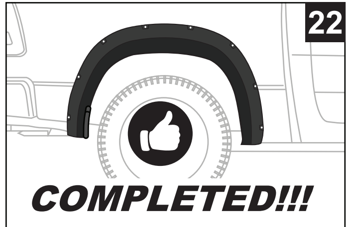
22. Tightly press flare against vehicle to evenly remove space between flare and vehicle. Tighten all 10 screws. Installation complete.
