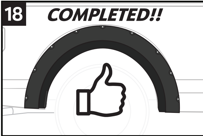
18. Tighten all screws. Repeat STEPS 12 to 17 to install the driver side rear flare.
