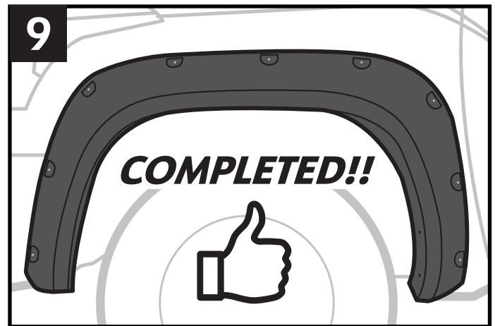
9. Make any additional adjustments to improve positioning of the flare. Follow the screw sequence number while tightening. Once finished, repeat STEPS 1 to 9 for the passenger side Fender Flare.
