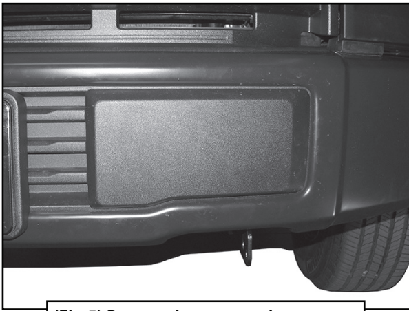
(Fig 5) Remove bumper pads to access splash guard hardware if necessary. Driver/left side of 2015 model F150 pictured
