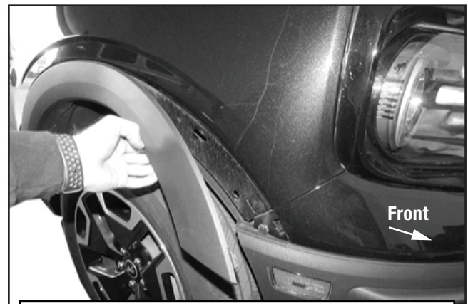
(Fig 4) Firmly pull the front end of the fender flare to release from clips. Only release front end of flare, do not remove flare
