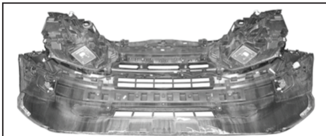
(Fig 12) Carefully remove the bumper cover assembly and place on a soft surface
