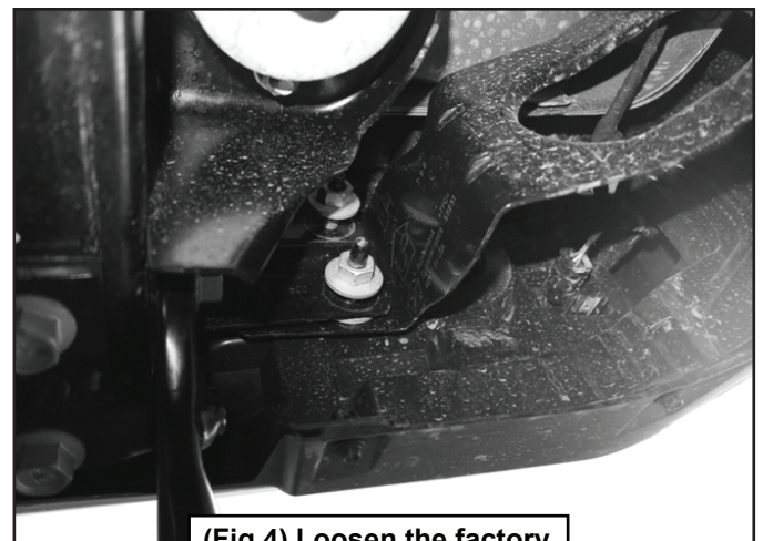
(Fig 4) Loosen the factory bumper bolts, (2 per side).
