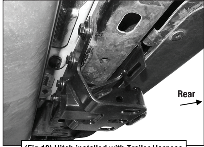
(Fig 10) Hitch installed with Trailer Harness Bracket on model with steel bumper option
