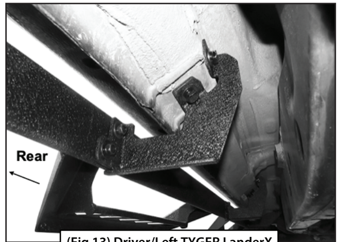
(Fig 13) Driver/Left TYGER LanderX attached to Rear Bracket (B)
