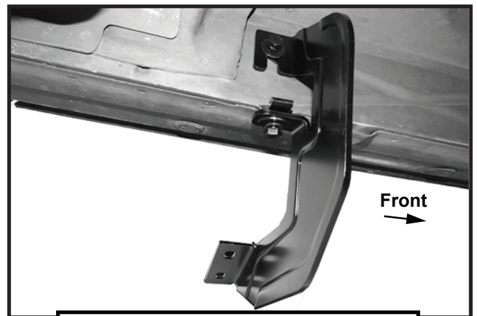
(Fig 21) Driver Side Center Bracket [A] attached
