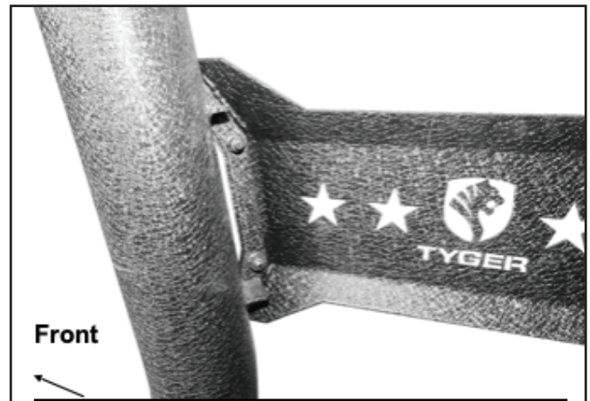
(Fig 8) Passenger/Right Decorative Plate installed
