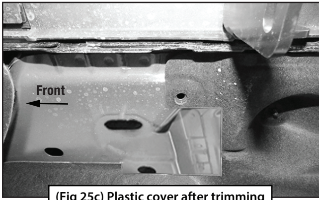
(Fig 25c) Plastic cover after trimming
