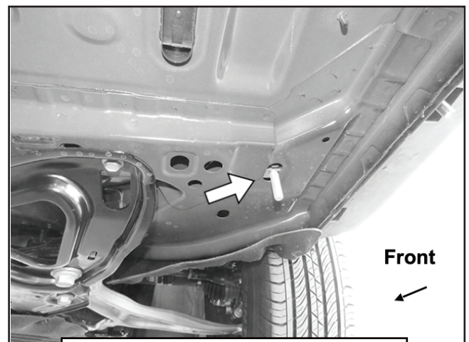
(Fig 11) Insert “Long” Bolt Plate into oval hole in front floor location (arrow)
