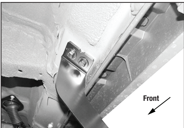
(Fig 7) (1) Passenger/Right Center/Rear Mounting Bracket attached to the 3rd location
