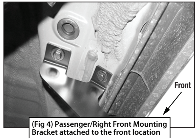
(Fig 3) Attach the Passenger/Right Front Mounting Bracket to the front location
