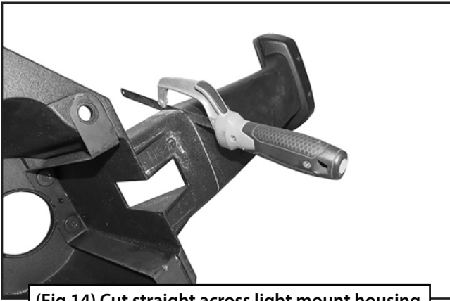
(Fig 14) Cut straight across light mount housing
