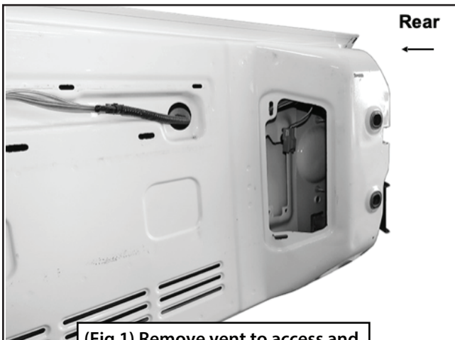
(Fig 1) Remove vent to access and unplug harness for 3rd brake light
